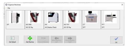
You can switch positions of machines and remove/add machines. In file menu you can import/export your machine setting and with "Set Default" you have a standard definition with all important machines.
