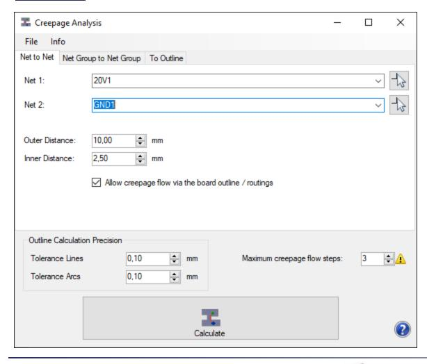
Net to Net creepage analysis is used to detect creepage issues between two single nets.
