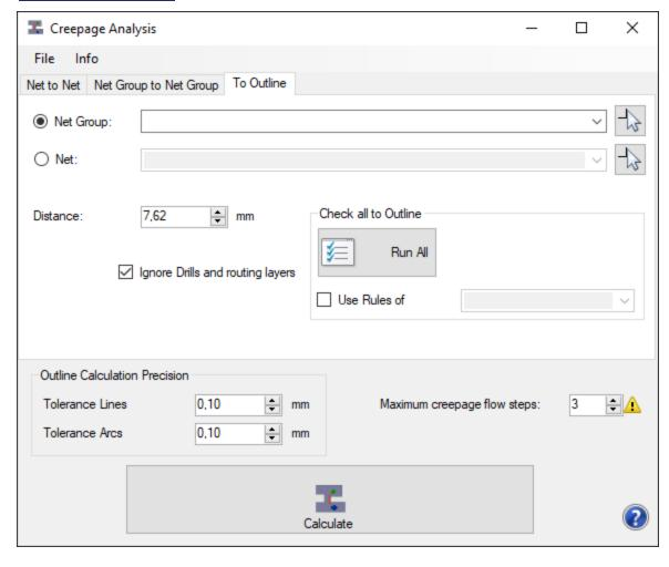
There is also an option to detect issues between a single net, or any net of a group to the board outline of the PCB
